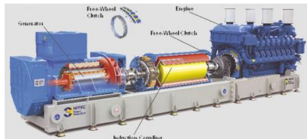
Figure 85 Rotating UPS
