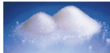
Granular aerogel: (sold under tradenames Nanogel, Lumira & Enova)
