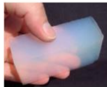
Monolithic aerogel (not available commercially)
