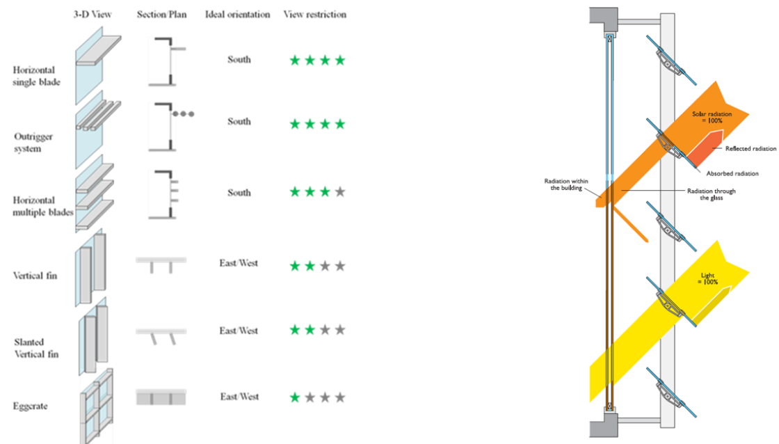
Above: Origination of solar radiation and simple shading optimal design. Source: BEMBook (IBPSA-USA) Below left: General types of horizontal and vertical exterior shading device. Source: BEMBook (IBPSA-USA) Below right: Shading louvers system. Source: MESTEK Architectural
