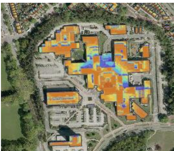
Figure 1.6 Solar radiation on the roof of Rijnstate Hospital in Arnhem
