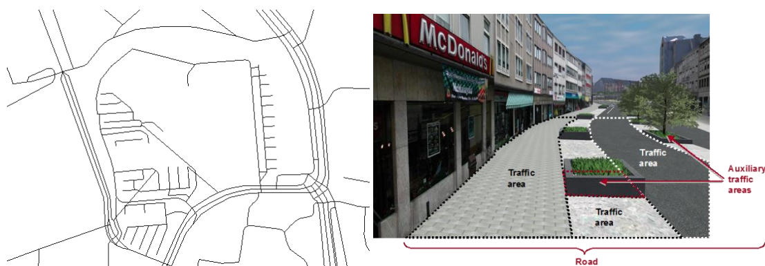
Figure 16: Roads of the Rijnstate hospital represented with LoD 0 geometry (left) and an example for a LoD 2 road, which is subdivided into different traffic areas (right) (source: City of Solingen, IGG Uni Bonn [CityGML2012])
